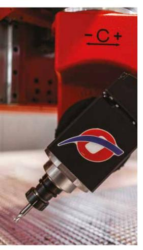
Electrospindle is one of the components most subject to wear or to accidental events that compromise its operation.
