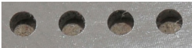
Figure 5. Drilled hole with no sign of defect.
