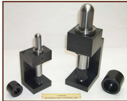
Compression Subpresses 1" and 2" Diameter ASTM D 695
