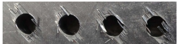
Figure 6. Drilled hole with delaminations and wear marks.
