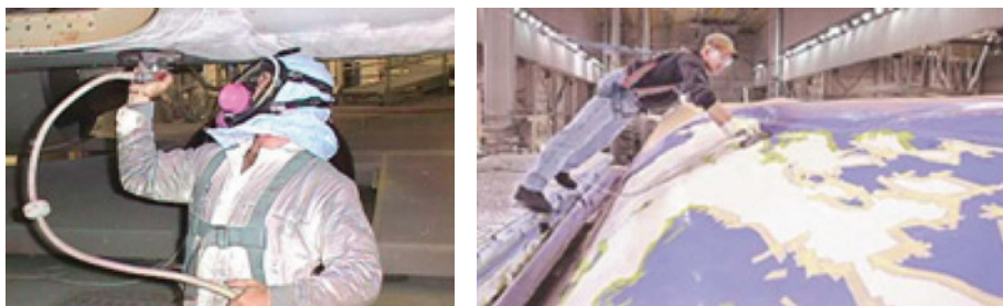
Figure 1. Mechanical abrasion to reactivate aged topcoat.
