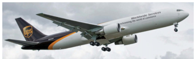
Figure 13. One of several UPS 767-300's that have received basecoat-clearcoat. Application of SM-1 is on the entire basecoat of the fuselage and empennage prior to clearcoat application. Photo (Boeing).
