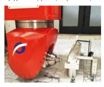
Heidenhain linear scales feedback systems with a 5 micron resolution on the linear axes and highly rigid frames, an enhanced machining accuracy and surface finish quality is achieved.
