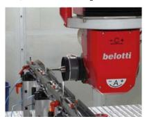
sweep of  $\pm 135^{\circ}$ . Productivity is assured with linear axes speeds of 50 m/min in X and Y, and 30 m/min in Z.
